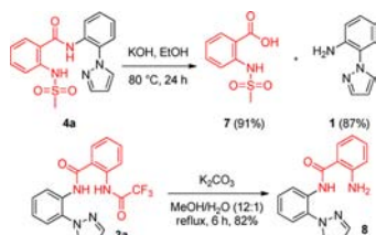
Scheme 5. A Possible Mechanism
