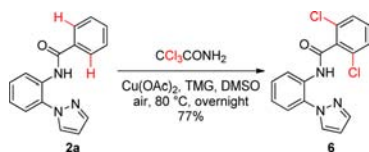
Scheme 3. Cu(OAc) 2 -Mediated Aerobic C(sp 2 –H) Dichlorination
